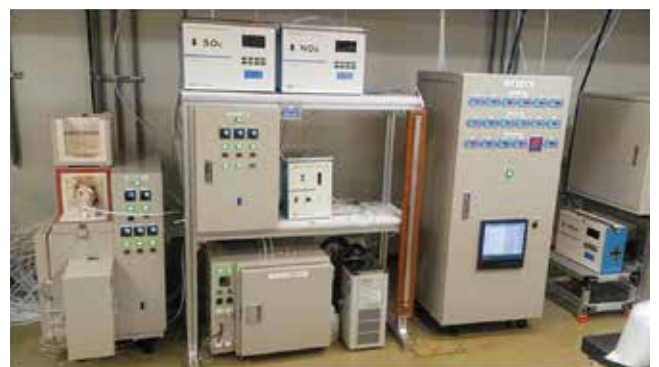
乾式脱硫性能評価装置 The evaluation system for efficiency of dry desulfurization
